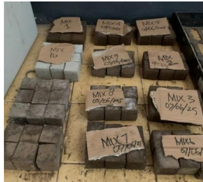
Figure 2. Ambient cured Geopolymer Speciment
